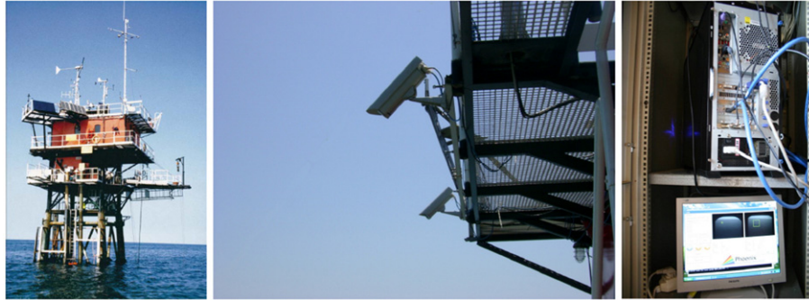
Fig. 1. Left: CNR-ISMAR oceanographic platform Acqua Alta off the Venice coast, Italy. Center: deployed WASS. Right: WASS data acquisition workstation.
